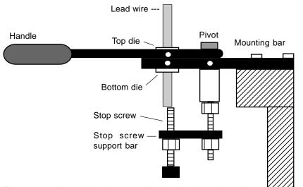
To remove dies, align the two dies in the closed position with the handle and mounting bar in a straight line. Then loosen the two set screws on the side of the bars, which
